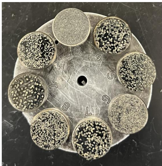
Figure 3. Samples were adhered to a carbon sticky dot and coated in a layer of carbon ~20 nm thick.
