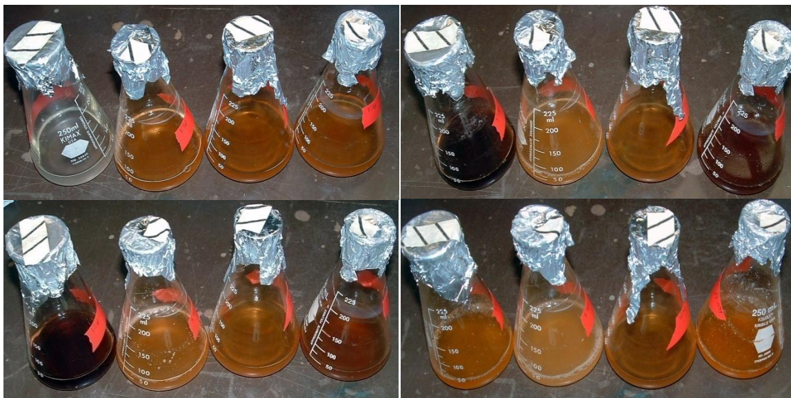
Figure 20. The four treatments shown in each photo above, from left to right, are Y. lipolytica AN-L15 and TNT (YT), Y. lipolytica AN-L15 and ferrihydrite (YF), ferrihydrite and TNT (FT), and Y. lipolytica AN-L15, ferrihydrite, and TNT (YFT). The top left photo shows the four treatments at the beginning of the experiment. The top right photo shows the treatments at thirty hours. The red color of the medium for treatments YT and YFT was indicative of the presence of 3-H-TNT. The bottom left photo taken at forty-two hours shows a change in color in the YFT treatment from red to orange this was indicative of the presence of a dihydride-Meisenheimer and protonated dihydride-Meisenheimer complexes. The change in color of the media from red to yellow, in treatments YT in the bottom right photo, was indicative of the presence of a dihydride-Meisenheimer and protonated dihydride-Meisenheimer complexes.
