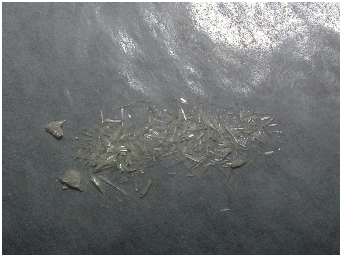
Figure 1. 2,4,6-trinitrotoluene in its crystalline form. This TNT is 99% pure thus giving a clear coloration to the crystals; less pure TNT often has yellow crystals.
