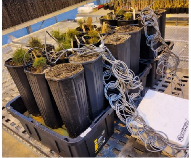
Figure 2: Diagram (A) and photo (B) of drought treatment method. Pots of juvenile trees (a) are on top of floral foam blocks (b) that draw up water from the bottom of the bin (c) to the pots. (d) is the distance between the top of the foam block and the surface of the water level, (e) is the distance between the bottom of the bin to the surface of the water level, and (f) is the soil moisture sensor.
