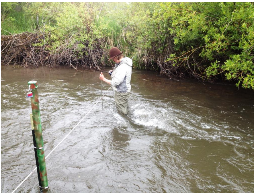
Figure 24. Measuring crosssectional area and velocity of Bozeman Creek at the BC1 gauging station.
