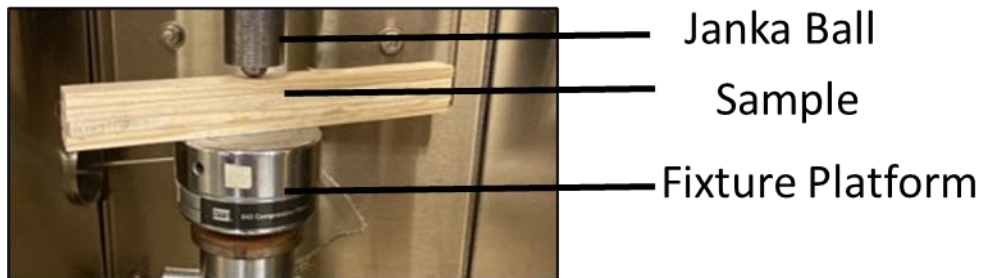
Figure 13. Hardness Test Setup
