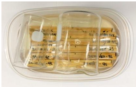
Figure 6. Delignification of Southern Yellow Pine Wood
