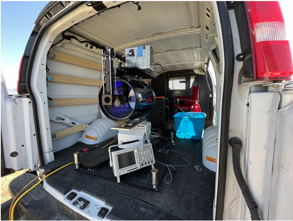
Figure 2.1: Photographs of the lidar system used to collect the training and testing data. This photo is courtesy of Trevor Vannoy
