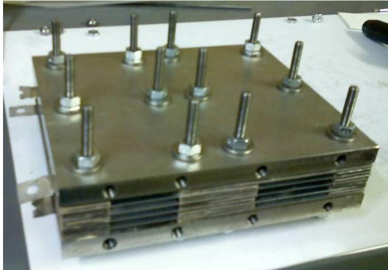
Figure 24: Fully-Assembled SSP with 10-32 Titanium through Rods
