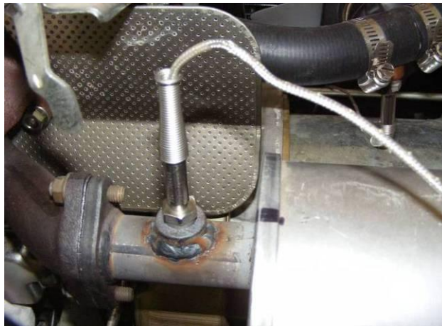
Figure 34: Thermocouple at Muffler Inlet
