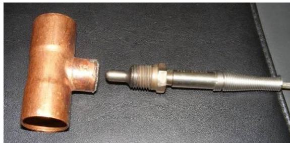
Figure 31: Pipe-plug Thermocouple and Fitting
