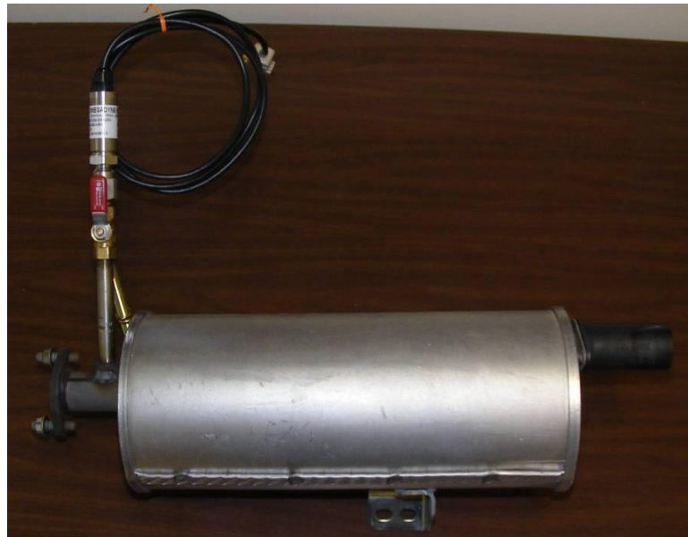
Figure 35: Stock Muffler with Pressure Transducer
