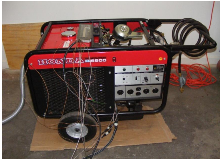
Figure 36: Instrumented Stock Honda ES650
