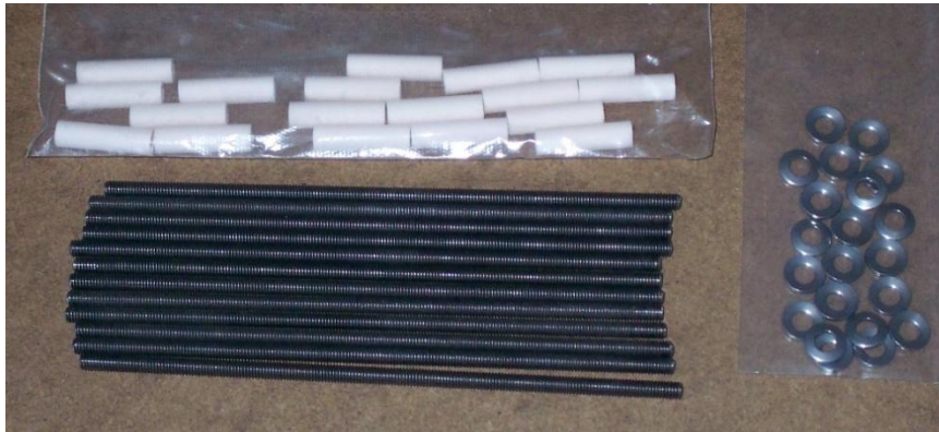
Figure 22: 10-32 Titanium Rods, Al 2 O 3 Tubes and #10 SS Bellevilles
