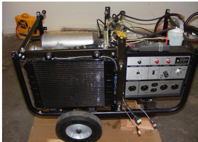
Figure 37: Instrumented ES650 with Panels and Fuel Tank Removed
