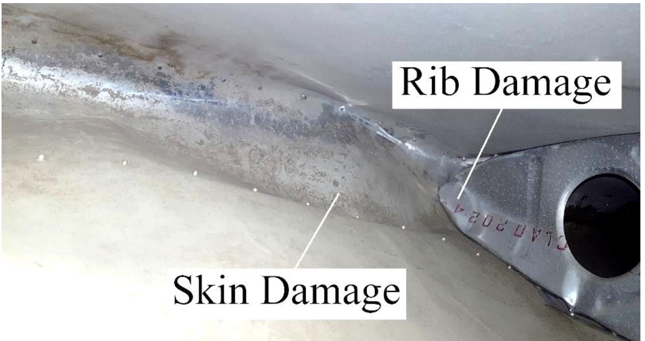
Figure 49. Interior Damage from Test 4
