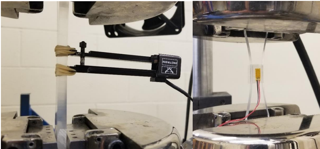
Figure 4. Tensile testing setup with an extensometer (left) and a strain gauge (right).
