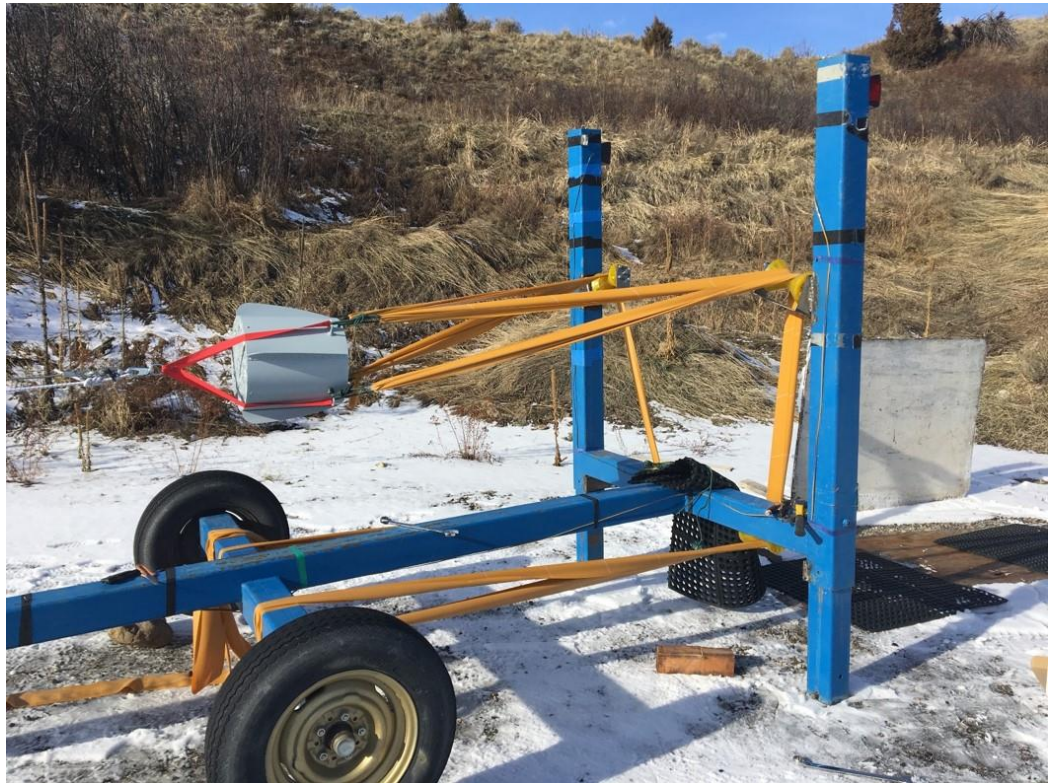
Figure 33. Compound slingshot design
