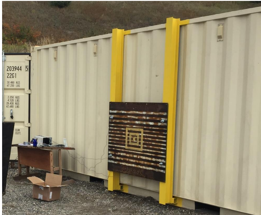
Figure 35. Shipping container impact tower with the 0.25” thick steel plate mounted
