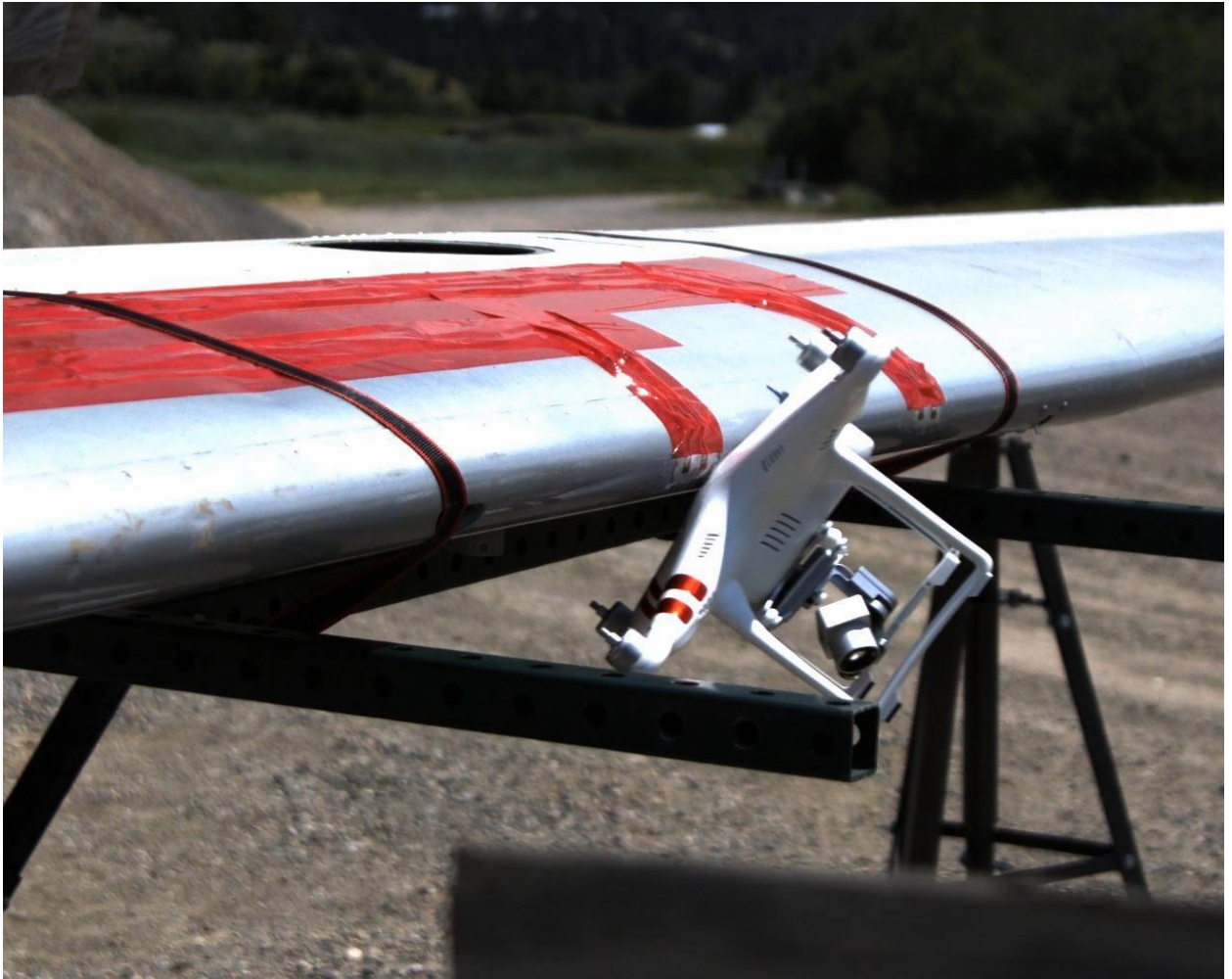
Figure 39. Impact orientation recorded with high speed video
