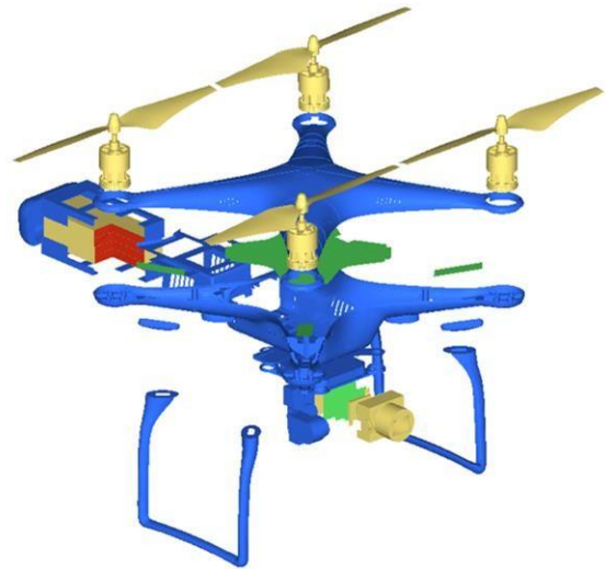
Figure 55. Exploded view of the DJI Phantom 3 model developed for LS-DYNA at NIAR [19]
