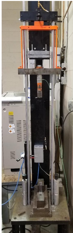
Figure 5. Impact tower setup for testing
