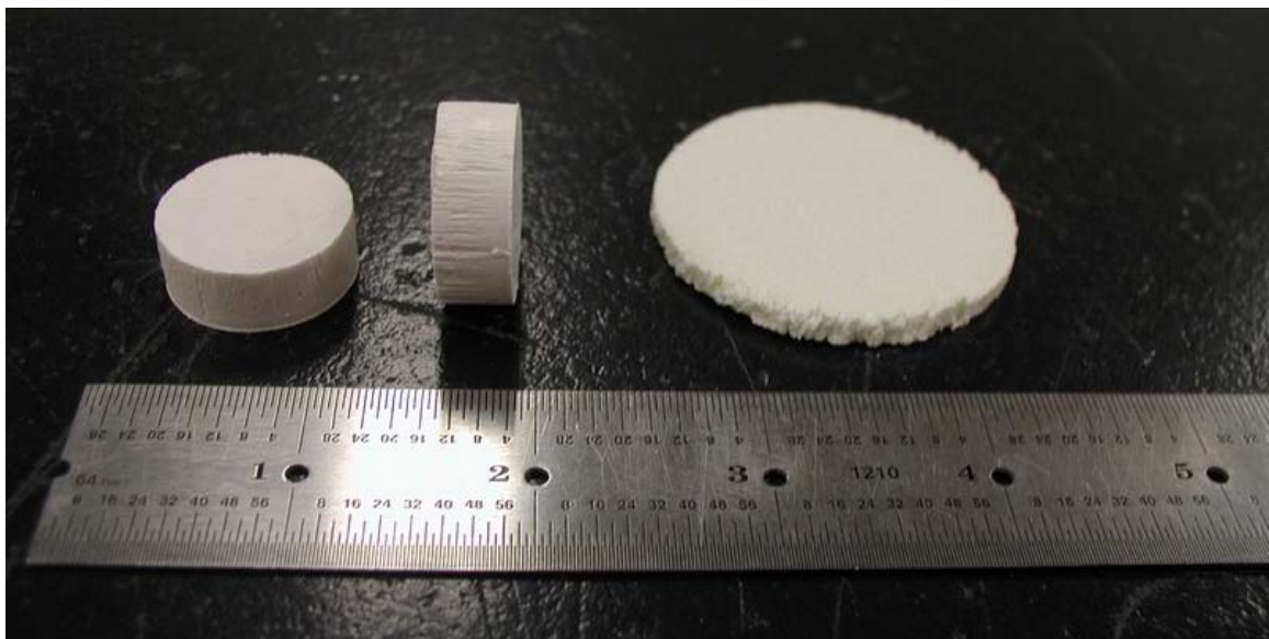
Figure 30. Two Die Cast (Left Half) and a Punched, Thick Freeze-Tape Cast (Right) Sample.
