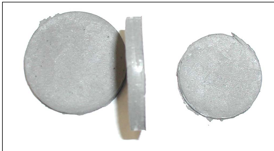
Figure 31. Captive Die Freeze Cast of Stainless Steel.
