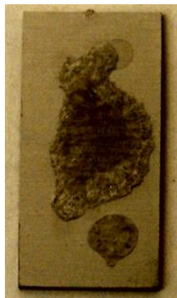
Figure 19: Photo of a sample coupon with a deposit of \sim 1 \frac{mg}{cm^2} of Na 2 SO 4 .
