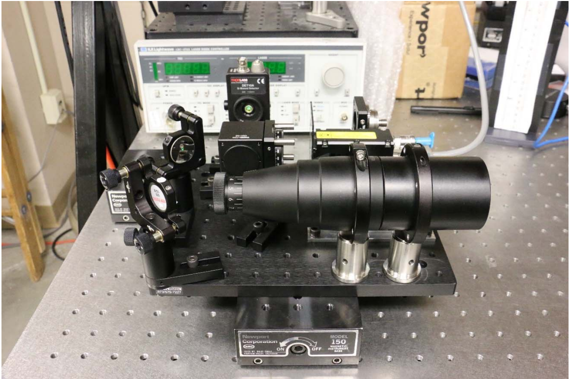
Figure 4.6 MPL transmitted beam collimating procedure performed in the lab.
