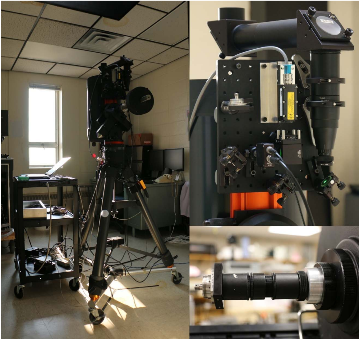
Figure 4.3 MPL system (left), transmitter (top right), and receiver (bottom right).
