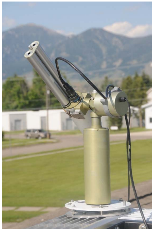
Figure 1.4 CIMEL sun sky multiband photometer model CE318-N at Montana State University, Bozeman site 45.67°N 111.05°W. (Picture courtesy by Joseph Shaw, Montana State University)
