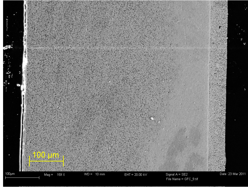
Figure 6.7: SEM image showing the lack of any discernible irreversible degradation in the fuel cell used to achieve EIS measurements during load-driven degradation and recovery.
