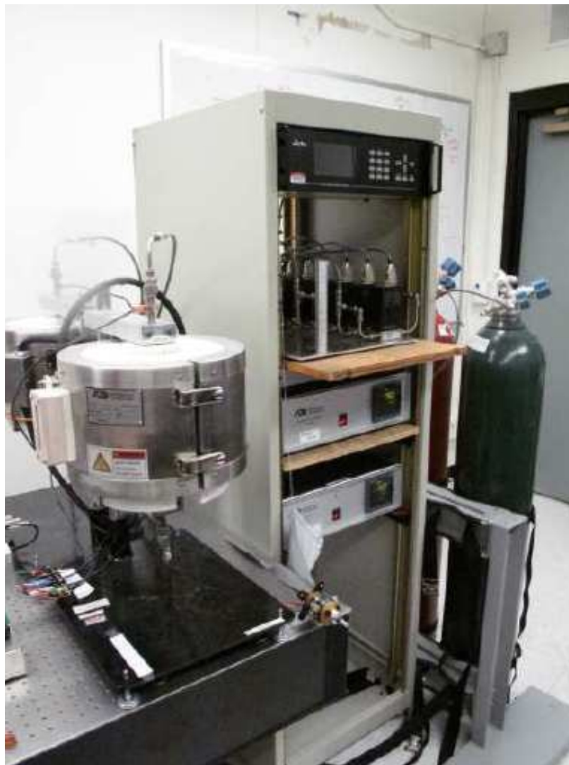
Figure 2.6: Gas delivery system and temperature control system for solid oxide fuel cell testing.
