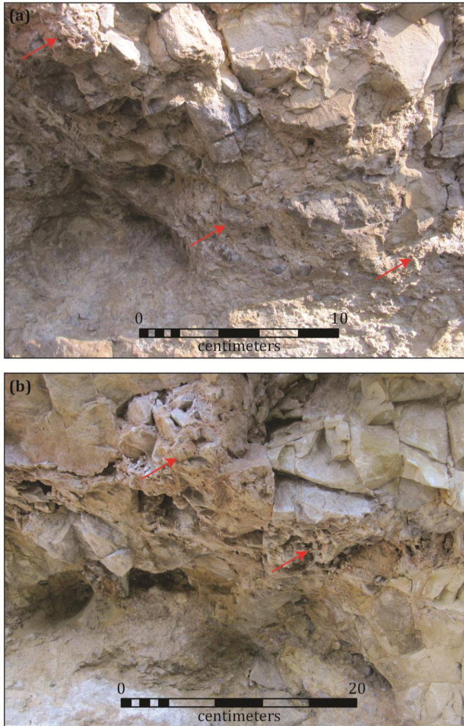
Figure 18. Outcrop photograph exhibiting the internal heterogeneities within a breccia pipe. The field outcrop photographs (a and b) of breccia pipe BSM-020 along the BSFS show zones of more intense brecciation and alteration, as indicated by the red arrows. These areas are interpreted to have been more permeable conduits for fluid flow during previous reactivation events.
