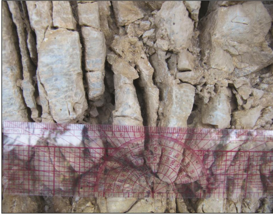
Figure 26. Outcrop photograph of fracture density and aperture in an argillaceous unit. This close-up of fracture station BSM-019 E along the BSFS is of fractures that are located in a more argillaceous unit, exhibiting a higher fracture density and larger aperture than was present in the more massive crystalline limestone that composes most of the Mission Canyon Formation.
