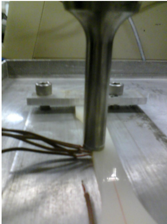
Figure 21: Picture of the Nylon dog bone sample with thermocouples imbedded and ultrasonic probe applied.
