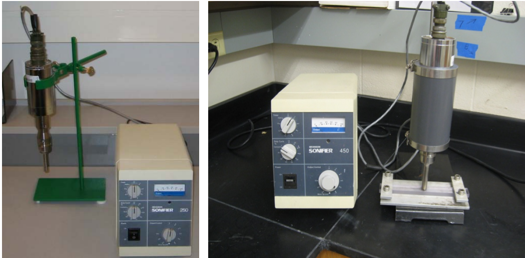
Figure 20: Comparison of old ultrasonic probe stand and the new stand machined for more precise alignment between probe and specimen.
