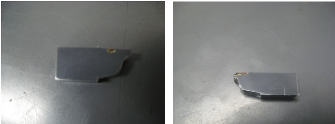
Figure 49: Damage caused by ultrasonic probe operating at various power levels. Left: Power Level 4 (160 W) generally localized damage not always over crack location. Right: Power Level 8 (320 W), higher power settings cause more wide spread damage.
