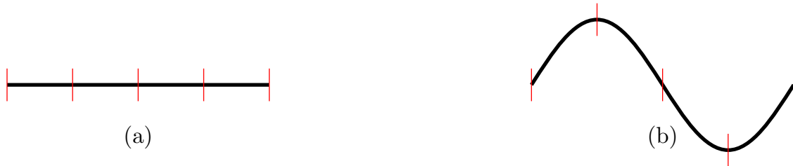
Figure 4: Effect of deformation on a discretized bounding wall. (a) Planar wall with evenly spaced nodes. (b) Sinusoidally deformed wall where nodes follow the shape of the deformation.
