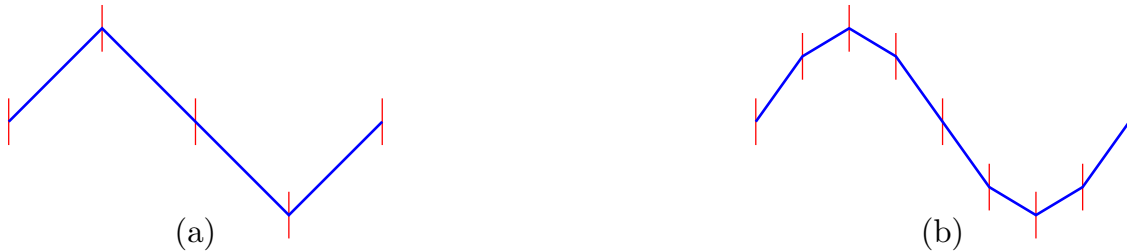
Figure 5: Comparison of coarse (left) and fine (right) meshing for DEM wall discretization. Finer meshing improves contact accuracy but increases computational cost. The red markers indicate nodal points used for contact detection, with finer meshes capturing more accurate wall deformations.
