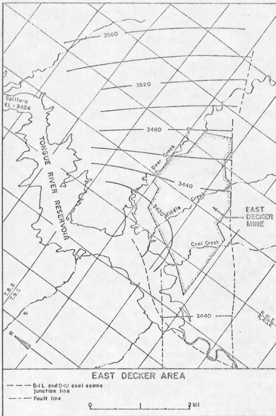
Fig. 27. Piezometric surface contours of the D-2 aquifer produced by the pre-mining, steady state simulation.
