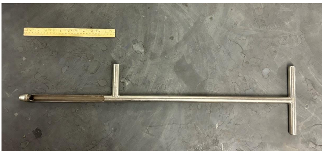
Figure 1.7. A standard push probe used to collect soil cores mentioned in Walter et al. (2016).
