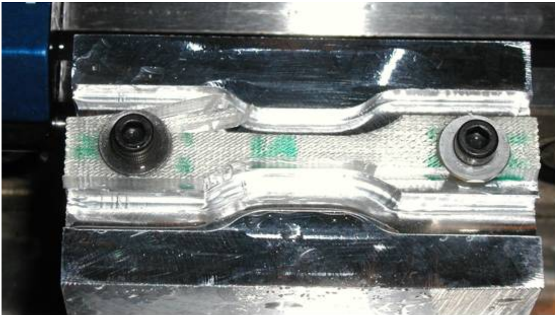
Figure 19. Delaminated tensile test specimen in the axial direction.
