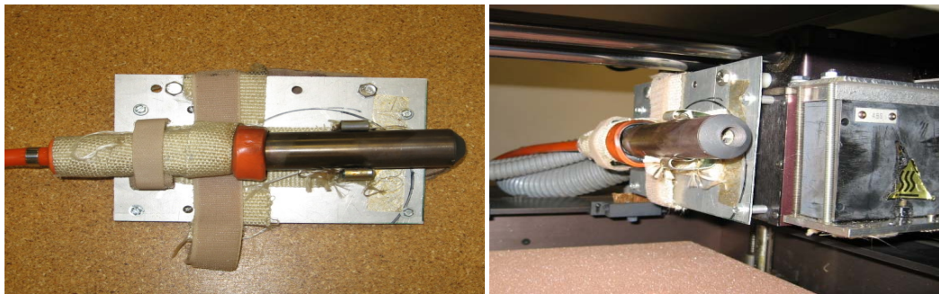
Figure 6. Welder and frame, unmounted and mounted configurations.
