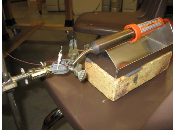
Figure 4. PVC welder temperature test setup
