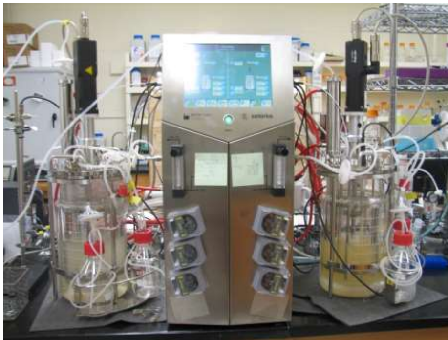
Figure A.13. Biostat B Twin Plus 5L jacketed reactors by Sartorius Stedim Biotech as seen under operation with temperature and stir rate control. Both reactors are filled with cultures of A. sarcoides .
