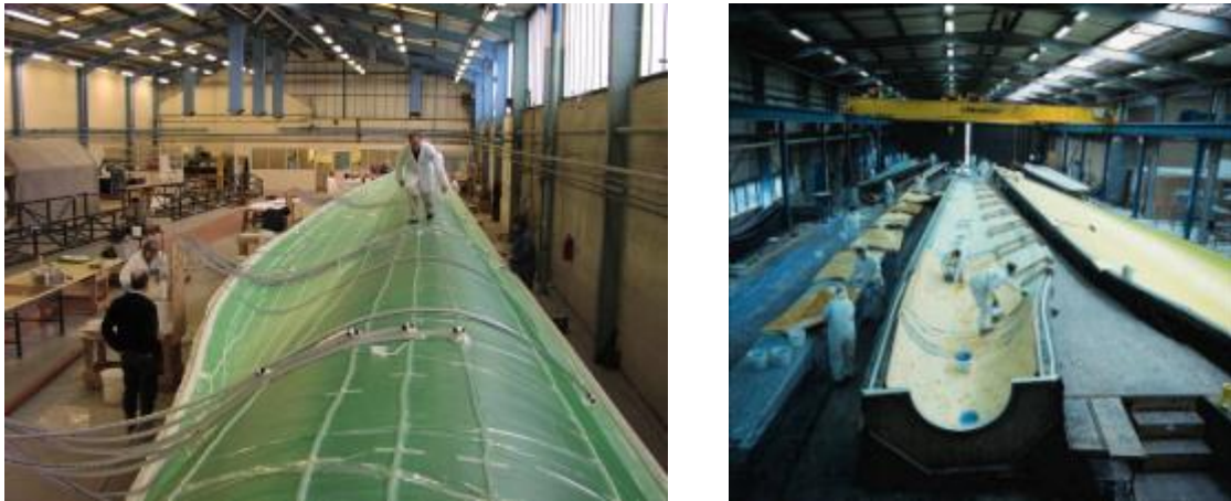
Figure 10. Hand layup of composite wind turbine blade [12]
