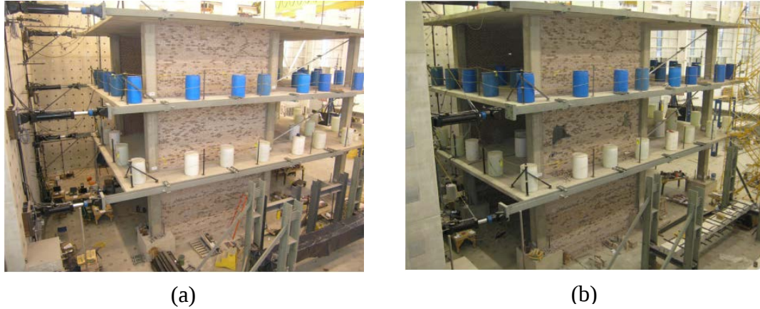
Figure 3: Three-story masonry infill test structure (left) before testing, (right) after testing (Pujol and Fick 2010)
