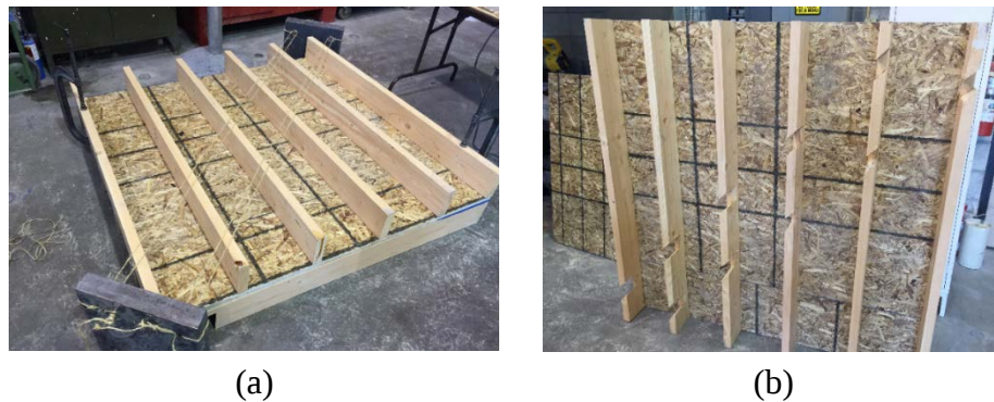
Figure 20: Platform construction for wall specimens. (a) creating holes for tension rods to pass through underneath the specimens and (b) completed platform
