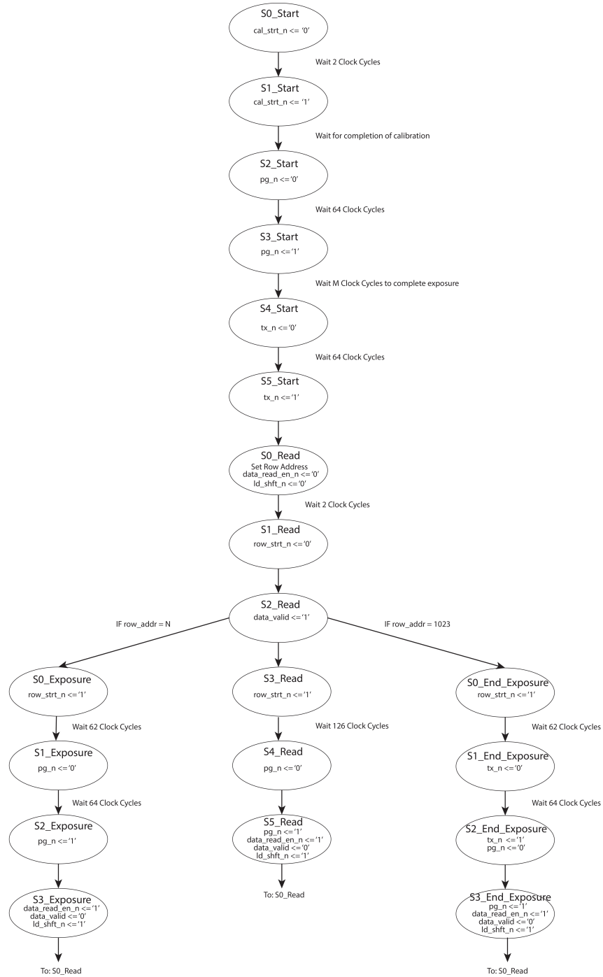
Figure 2.11: The Camera Control State Machine, showing the follow through the states and the output signals of each state.
