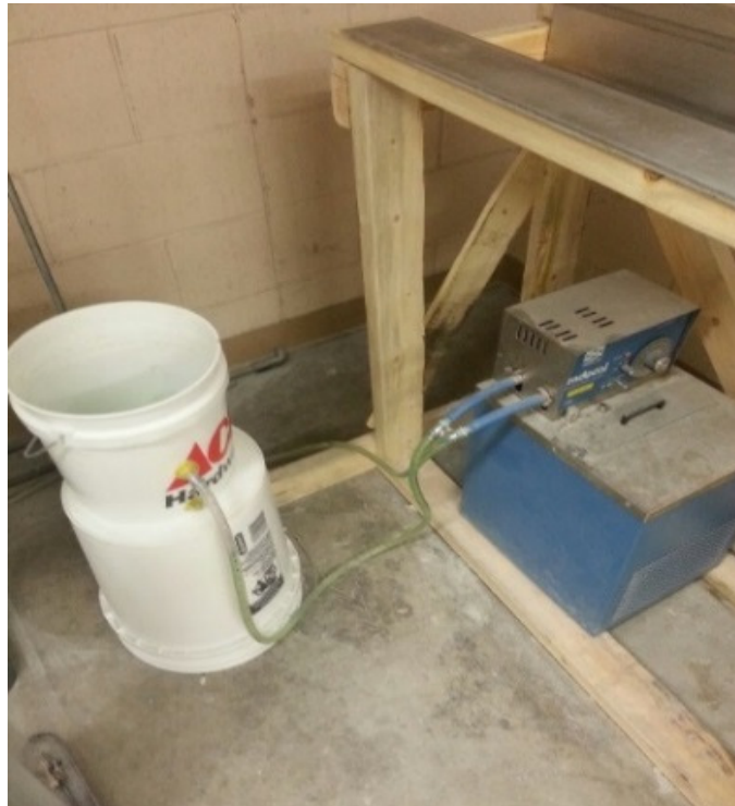
Figure 26 - Endocal Bath for Heating Resin
