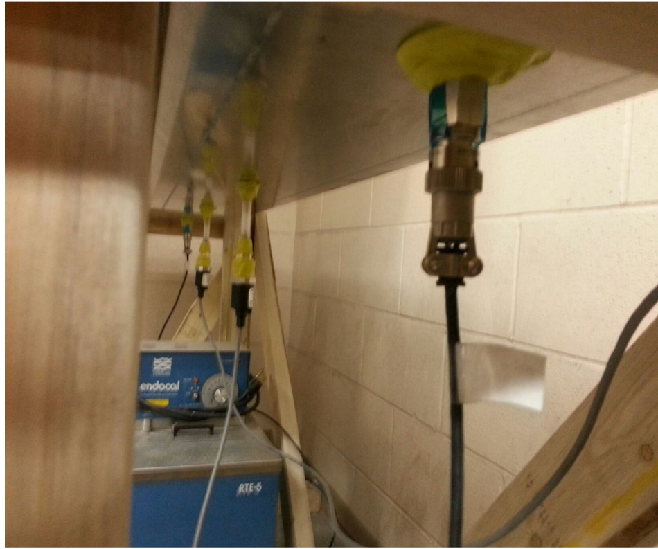
Figure 24 - Mold with Sensors Attached
