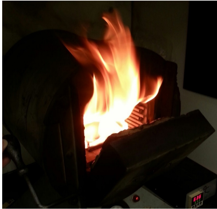
Figure 33 - FV Burn Off in Muffle Furnace
