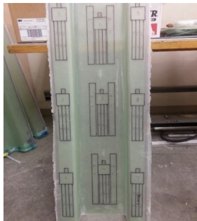
Figure 28 - Samples Taken from Beams
