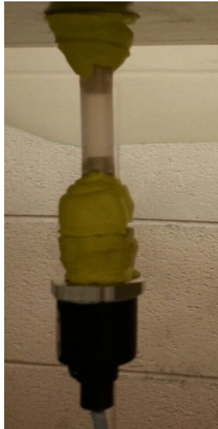
Figure 23 - Non-Flush Sensor Attached to Mold
