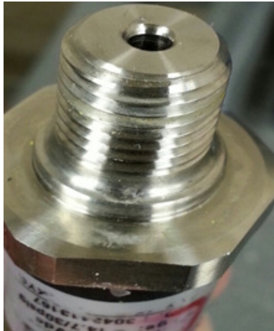
Figure 20 - Non-Flush Pressure Sensor
