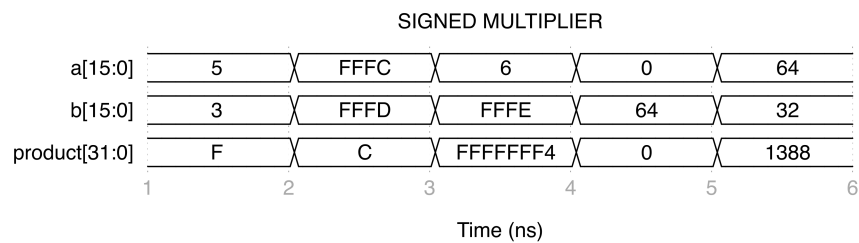
Figure 52: Timing waveform for 16-bit signed multiplier demonstrating multiplication operation.
