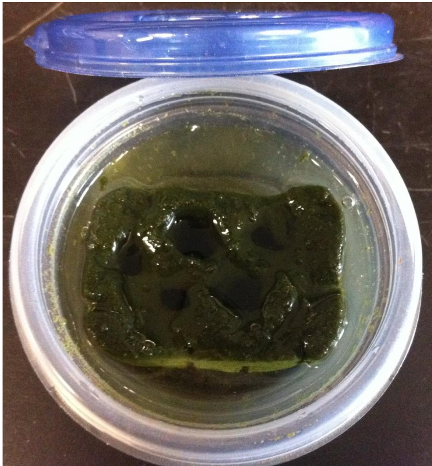
Figure 2. A humidifying container. It is made up of a plastic container with an air tight cover fitted with floral foam which was flooded with FAUP.
