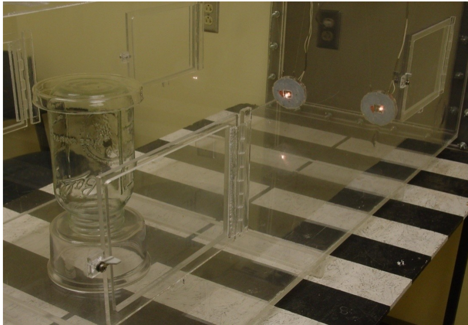
Figure 3.1. Wind tunnel apparatus used to test behavioral responses of B. cephi and B. lissogaster to synthetic compounds known to be produced by wheat plants infested by wheat stem sawfly.
