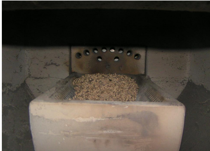
Figure 36: Burn chamber with pellets loaded
