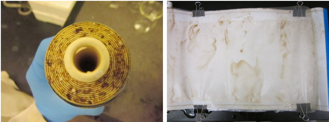
Figure 38: Phase III final autopsy images (Line 3). Left – The lead face of the membrane element. Chunks of solids and some biomass can be observed. Right – The membrane surface is visibly much cleaner than in combined and organics loading cases. Upon closer inspection lighter areas along the edges can be seen which indicates areas where no flux occurred. Flow direction is downward on the page.
