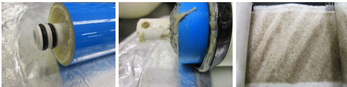
Figure 52: Phase IV combined and organics line autopsy photos. Left – Membrane telescoping observed in the combined line. Center – Membrane telescoping observed in the organics line and a great quantity of biomass on the front of the element and brine seal. Right – Fouling on the membrane surface of the organics line. The lighter colored areas along the edges are where flux does not occur. Flow direction is downward on the page.
