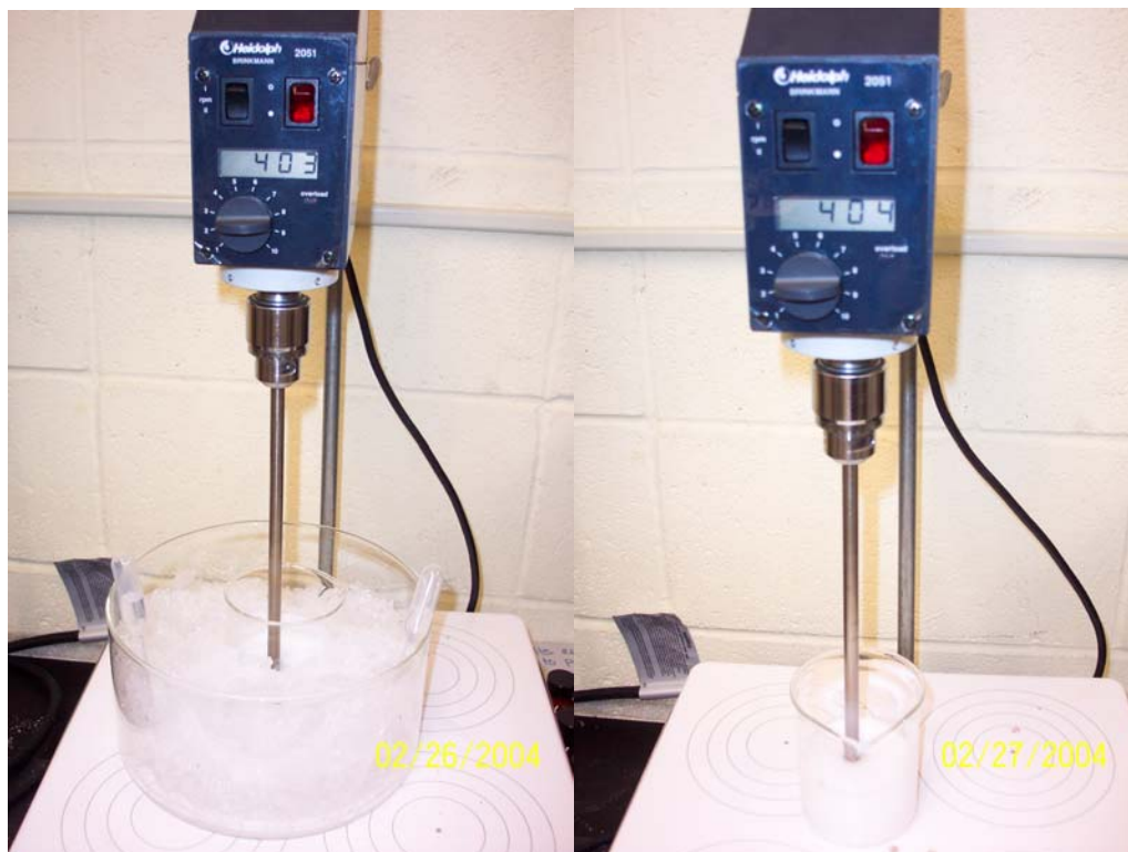
Figure 13. Salt Formation Test Setup: Ice Bath (Left); Hotplate (Right)
