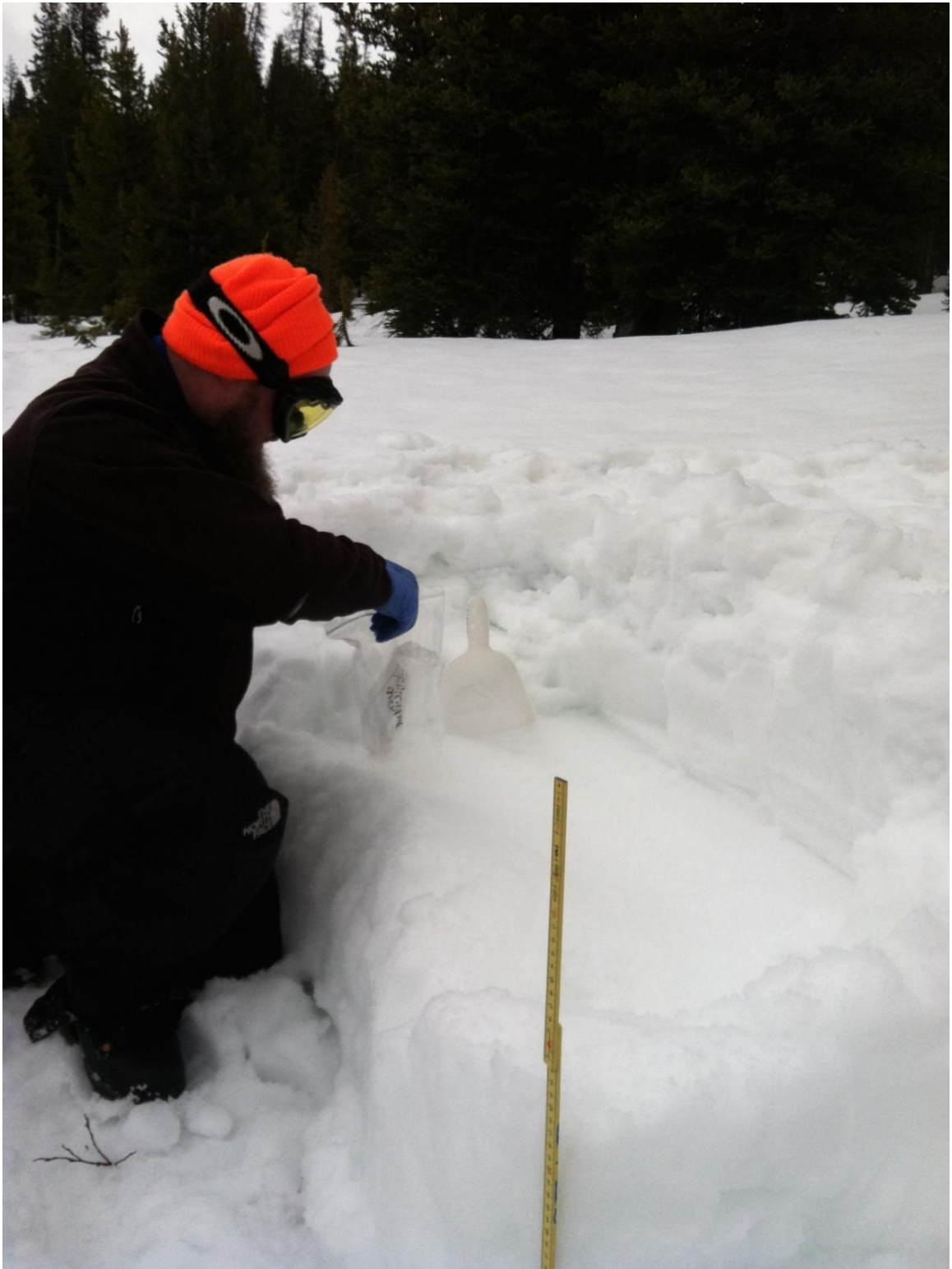
Figure 2.10. Sampling of isolated layers in the snowpack at Beartooth Lake, May 19, 2015. This was close to the peak snowpack for the 2014-2015 snow year.
