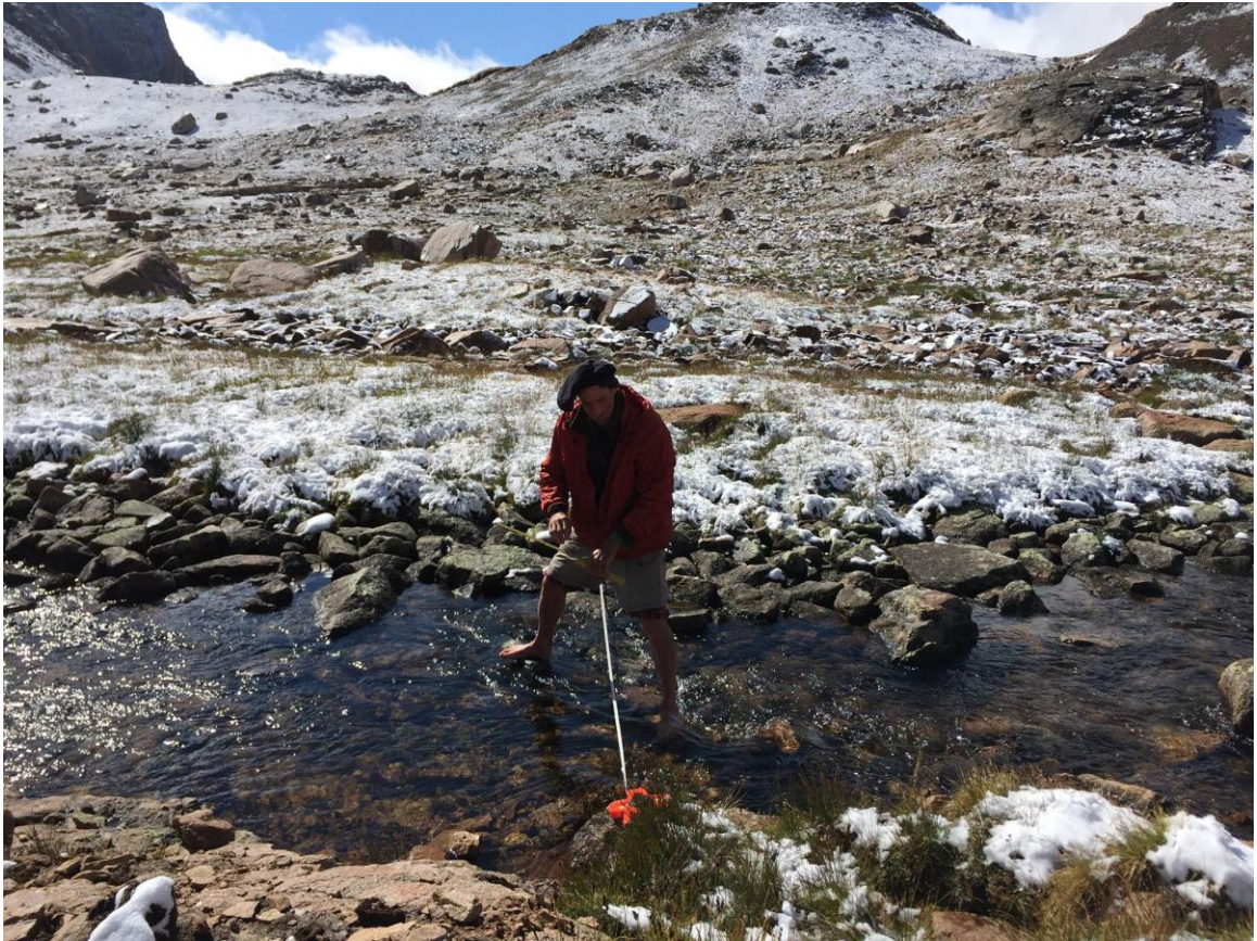
Figure 2.16. This is the same location as Figure 2.15 but looking due south, perpendicular to Figure 2.13. This photo was taken on August 25, 2016, DoY 238 after a significant snowfall (~7cm) the night prior. Here a field technician is performing measurements taking the cross-sectional area of the wetted perimeter.
