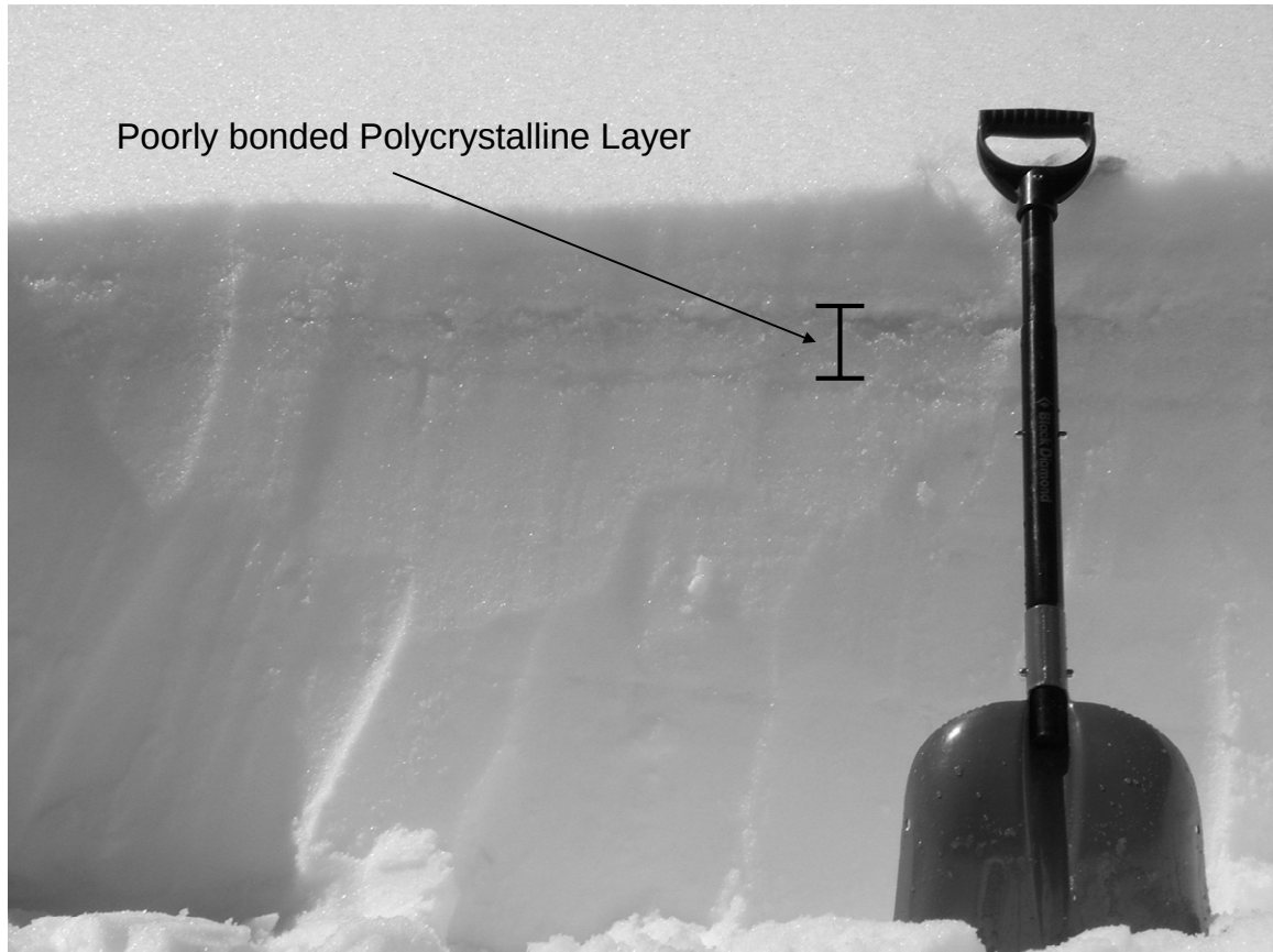
Figure 3.11. Atypical, weak polycrystalline layer involved in the 26 April 2004, wet loose snow avalanche (please refer to Figure 3.12 for stratigraphy related to this picture).
