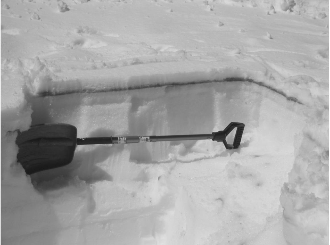
Figure 3.4. Melt-water accumulation, or 'horizon' along a surficial stratigraphic interface. Powdered dye was applied to the surface prior to the daily melt cycle.
