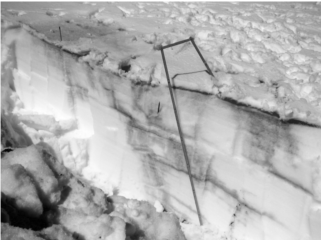
Figure 3.6. Melt-water penetration to the depth of the snowpack. In this picture water initially accumulated along the well defined near surface layer (see Figure 3.4), until that layer was compromised (in this case a dog walked over the study plot). After the surface layer was compromised, dye immediately penetrated to depth.
