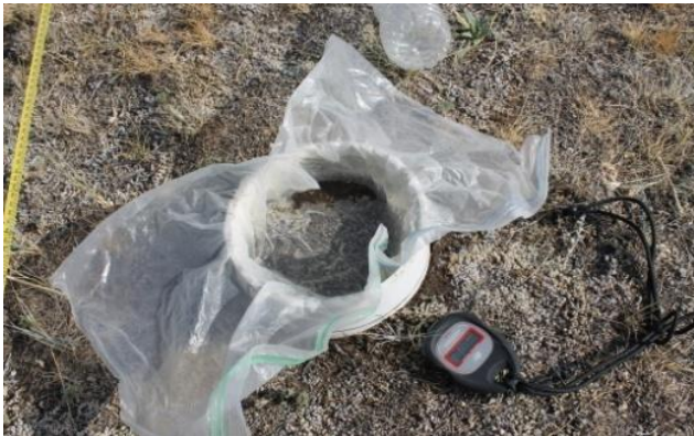
Figure 2. Photography of Single Ring Infiltrometer
