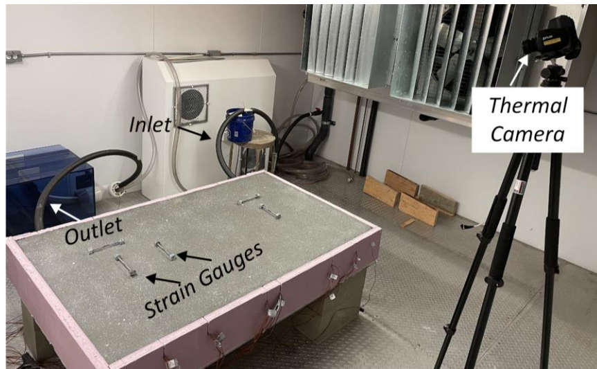
Figure 16: Bridge deck model prepared for testing
