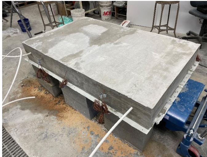
Figure 14: Cured bridge deck model
