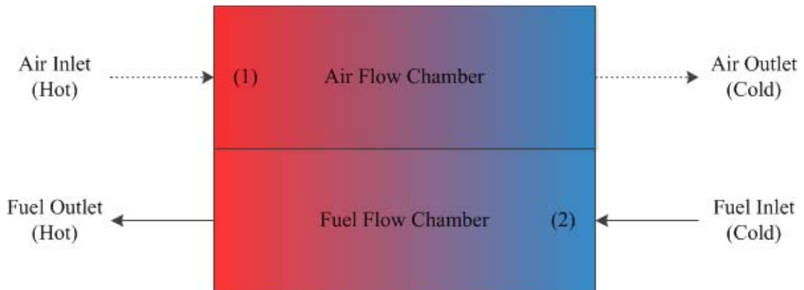
Fig. 2.33 General operation of a heat exchanger with air and fuel as inputs.
