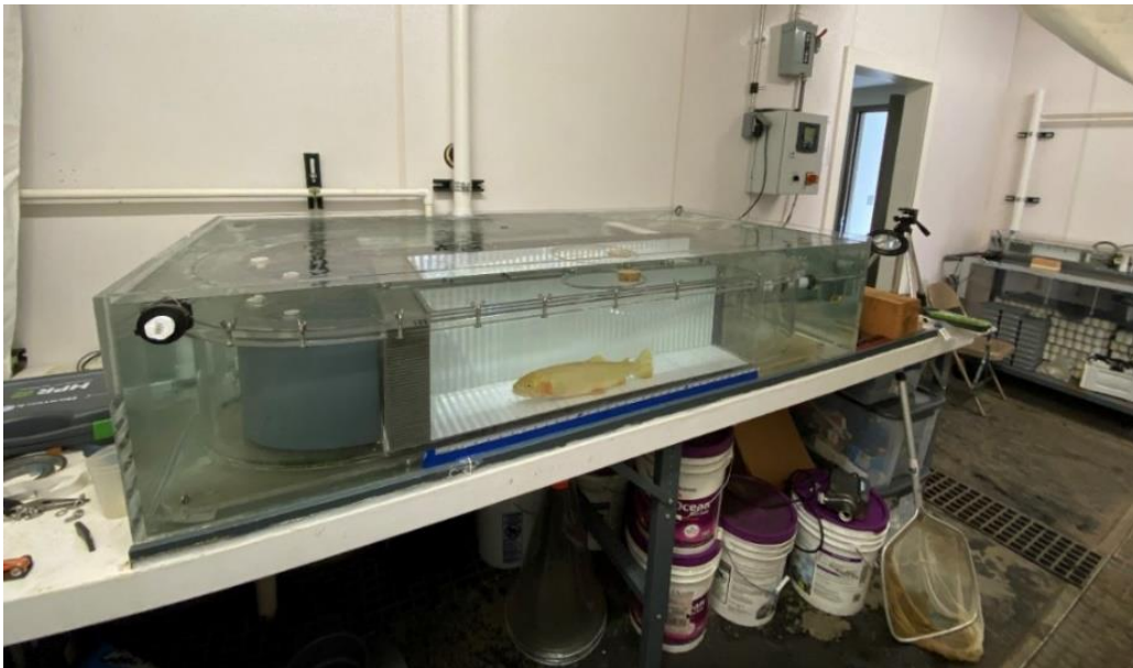
Figure 2.4: The swim chamber used to conduct the U_{\text{sprint}} experiment with a YCT in the test section.
