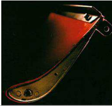
Figure 3. Gurney Flap Used on a 1971 Race Car 3
