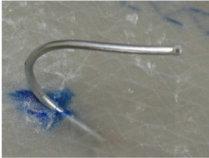
Figure 31. Aluminum Tube used as Fiber Optic Protector 30
