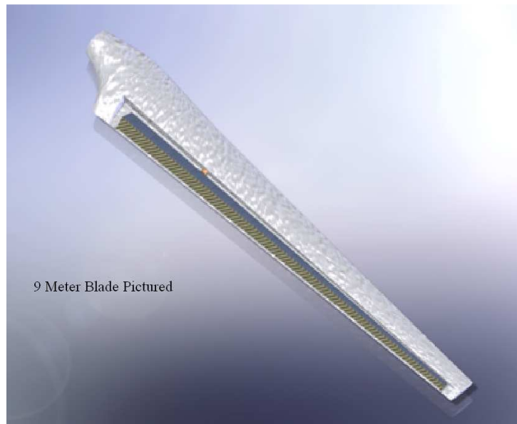
Figure 7. Gurney Flap Installed in Wing 7
