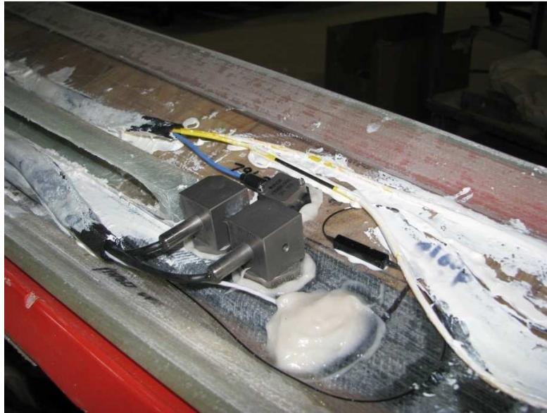
Figure 41. Sensors Affixed to the Inside of a Blade 40
