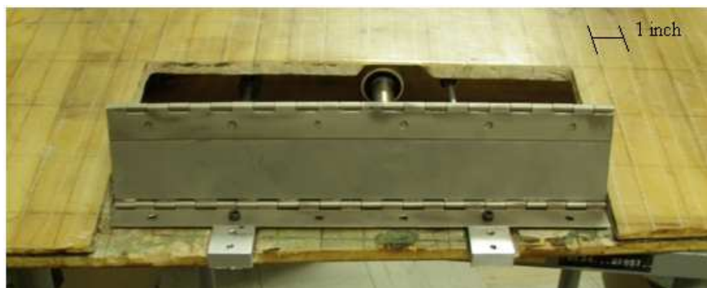
Figure 10. Gurney Flap installed in a Blade Section 9
