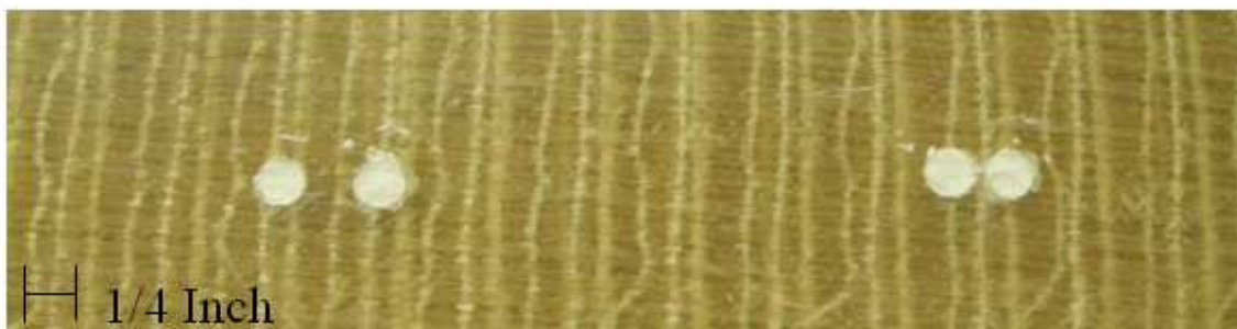
Figure 14. Recessed Holes Smoothed Over 13
