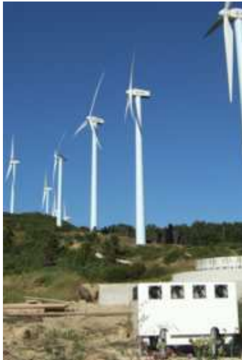
Figure 40. LIDAR Remote Measurement of Wind Profiles 39
