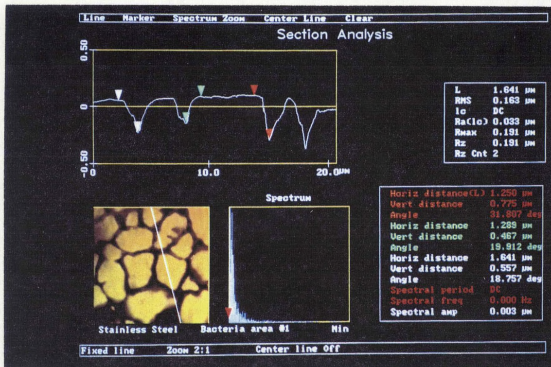
Figure 3. Section analysis generated by atomic force microscopy of the 316L stainless steel surface. Arrow color in upper left depth profile corresponds to vertical distance data in lower right.
