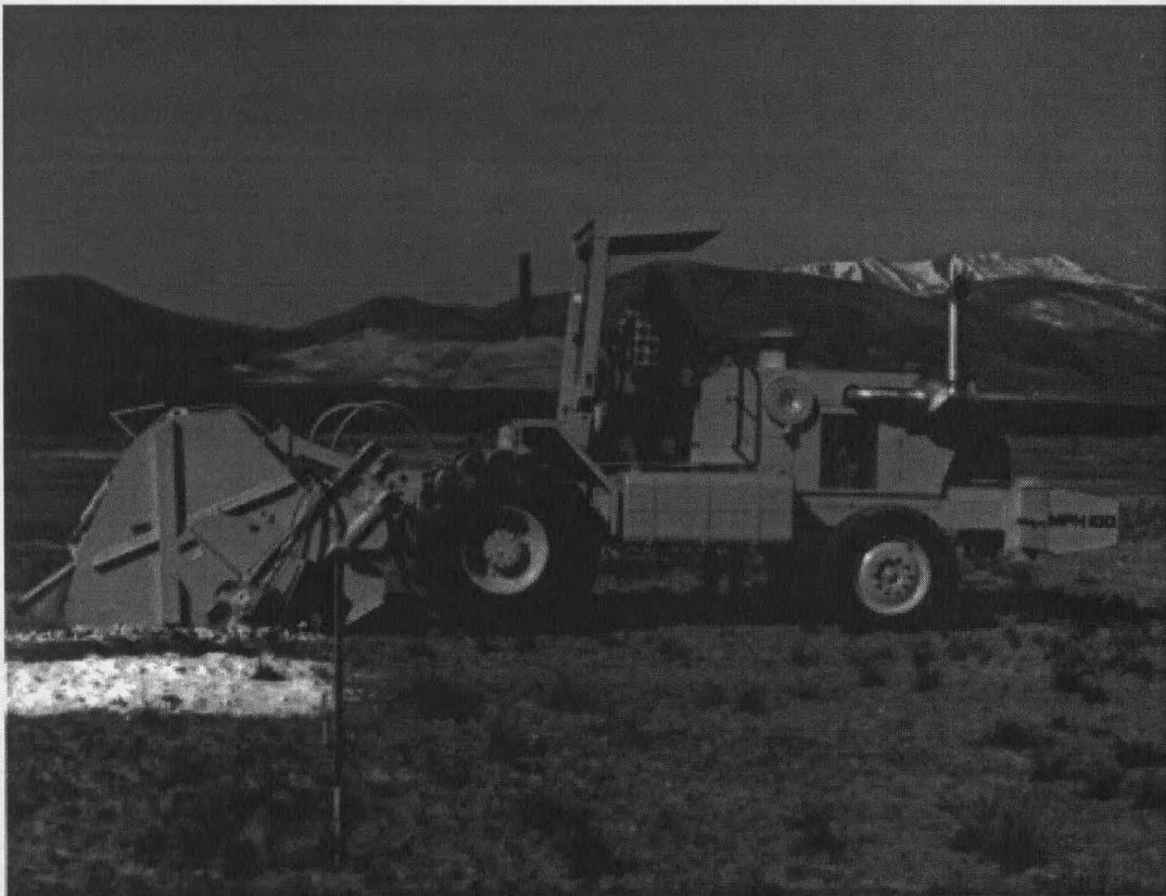
Figure 15. The BOMAG MPH 100 Soil Stabilizer rotary mixer.
