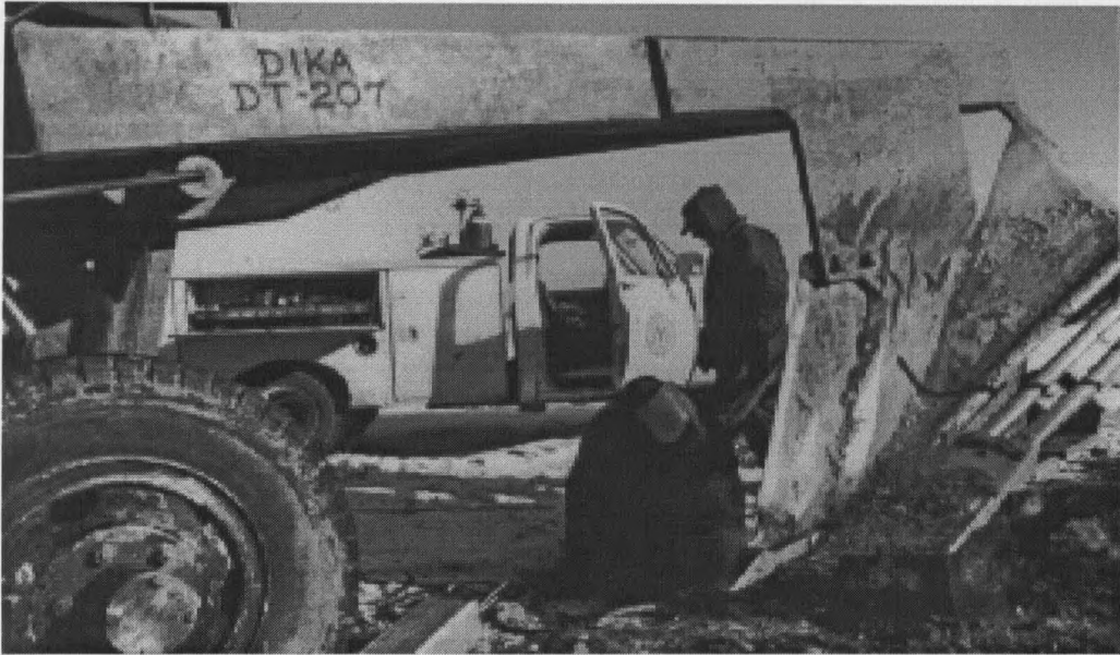
Figure 7. The Dika Plow can be used to plow soil to the 4 foot depth (Dollhopf 1992).
