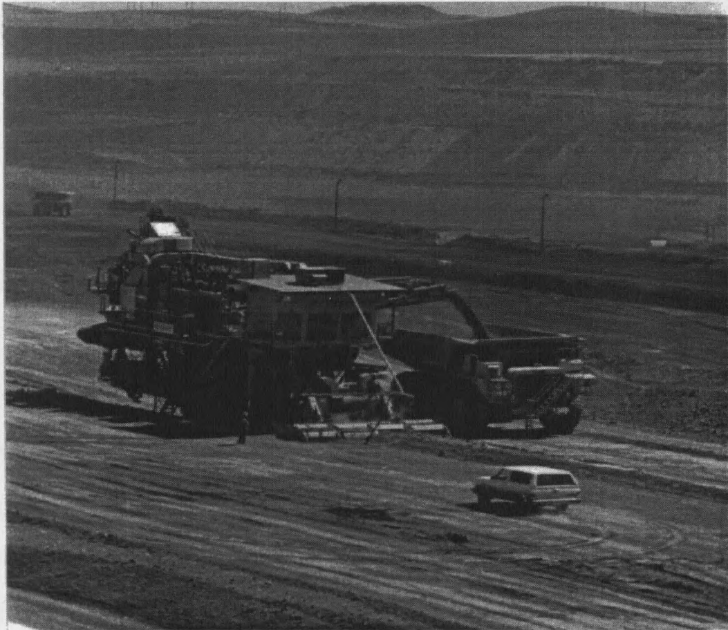
Figure 9. The Krupp KSM-2000 Surface Miner excavating minesoil into a haul truck.
