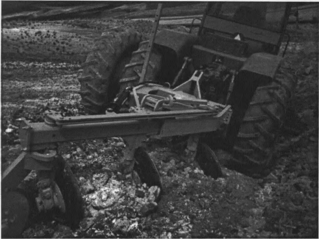
Figure 14. The Baker Plow with three mounted discs.
