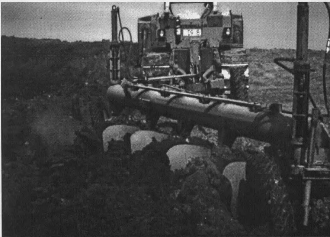
Figure 8. The Towner Plow with four moldboard plow shares (Dollhopf 1992).
