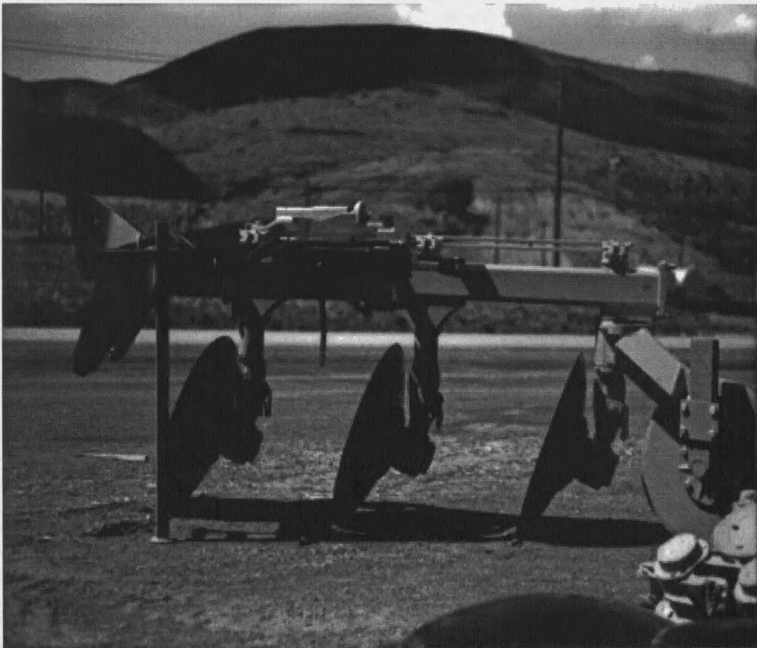
Figure 1. Baker Plow equipped with three discs.
