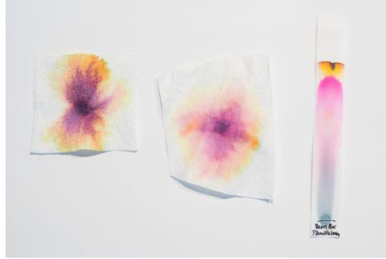
Figure 4. Black pen chromatography on various types of paper (Bosly, 2018).
