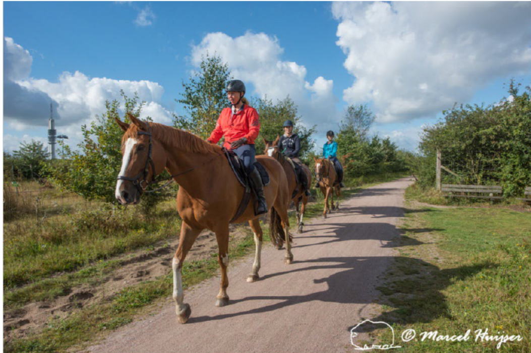
Figure 53. Horseback riders on a trail on a multifunctional overpass across a 2-lane road and railroad tracks. The trail is for non-motorized recreation. Natuurbrug Zanderij Crailoo, The Netherlands. The trail has a berm with trees and shrubs on the right-hand side to reduce human presence and disturbance in the wildlife zone that is further to the right. There is also a berm with trees and shrubs to the left of the trail, reducing visual and noise disturbance from vehicles towards the trail.
