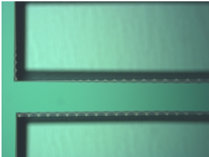
Figure 4.3: Large trench etched into silicon 120 \mu\text{m} deep
