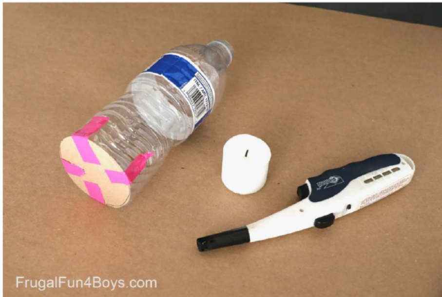
Figure 3. Plastic bottle with the bottom replaced now with cardboard and being flicked again to put out the flame with no air puff.
