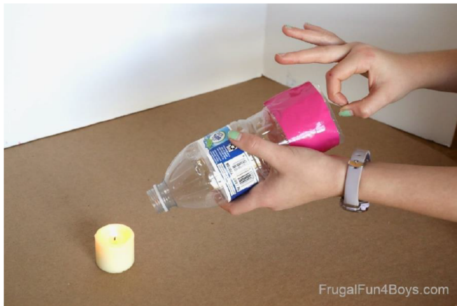
Figure 2. Plastic bottle with the bottom replaced with a part of a plastic baggie being flicked to put out a flame with sound waves.
