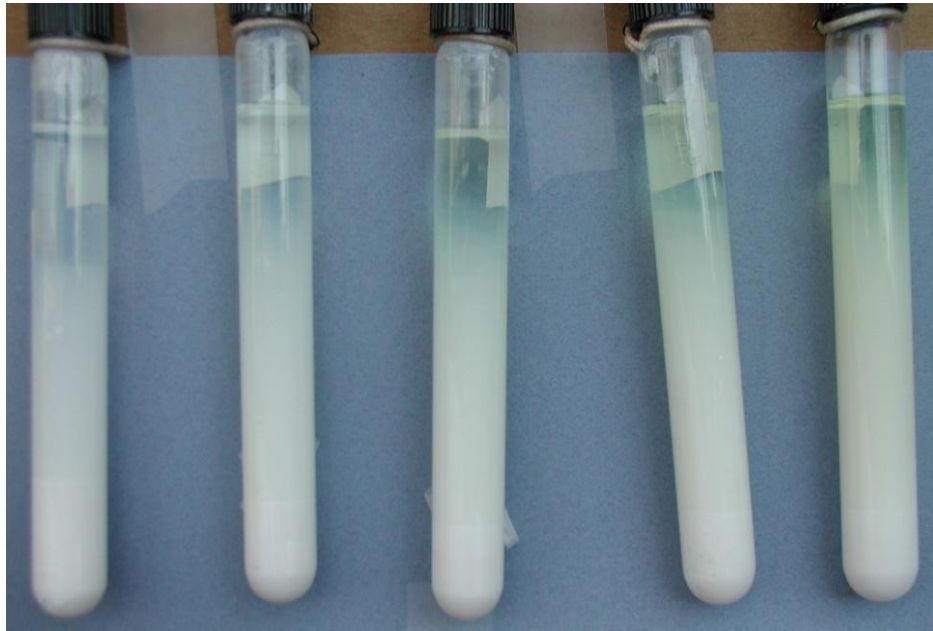
Figure 35. Centrifugal Test With 1-5% of MFO in 8YSZ in 1% increments (From Left to Right)
