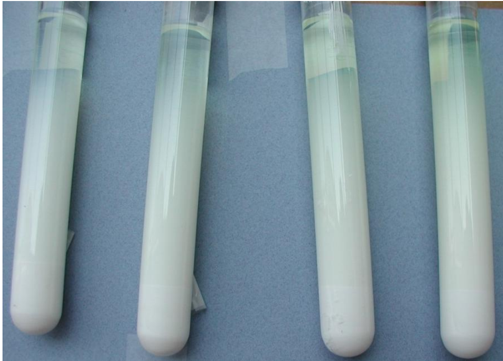
Figure 34. Centrifugal Speed Test with 8YSZ Slurry
