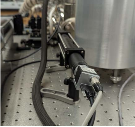
Figure 34: (a) The side camera is tilted to align the ‘transverse’ motion of the particle to the horizontal axis of the camera. (b) An image was taken by the tilted camera. The tilted configuration is aligned to the oscillation axes of the particle in the xy plane when the particle has accumulated excess charge. The dashed coordinate system represents the typical oscillation axes for a discharged particle; as charge accumulates, the axes begin to rotate, represented by the unprimed coordinate system in this image.
