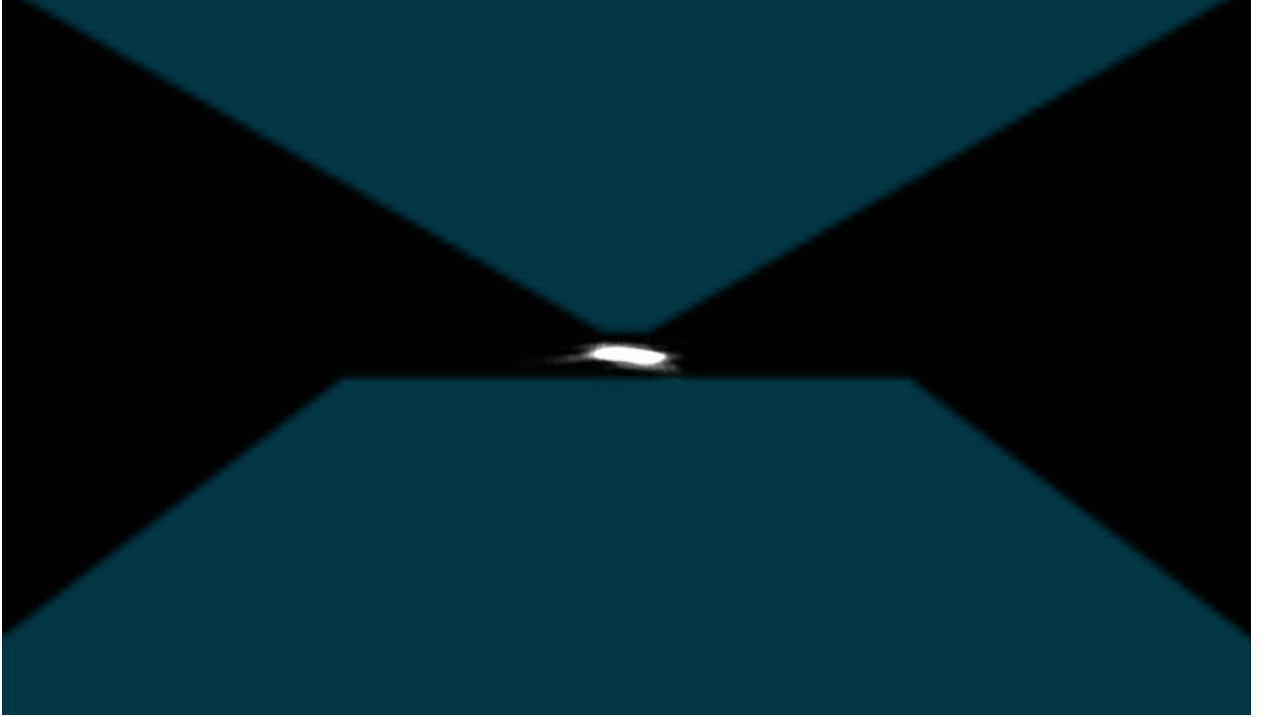
Figure 37: An image of the retro-reflector beam taken using the camera from Figure 36. An outline of the pole piece structure in this image is added for extra reference, but is not seen in the raw image file due to lack of exposure. In the center, the illumination beam returns through the trapping region after hitting our retro-reflector. This camera is needed for initial retro-reflection alignment.
