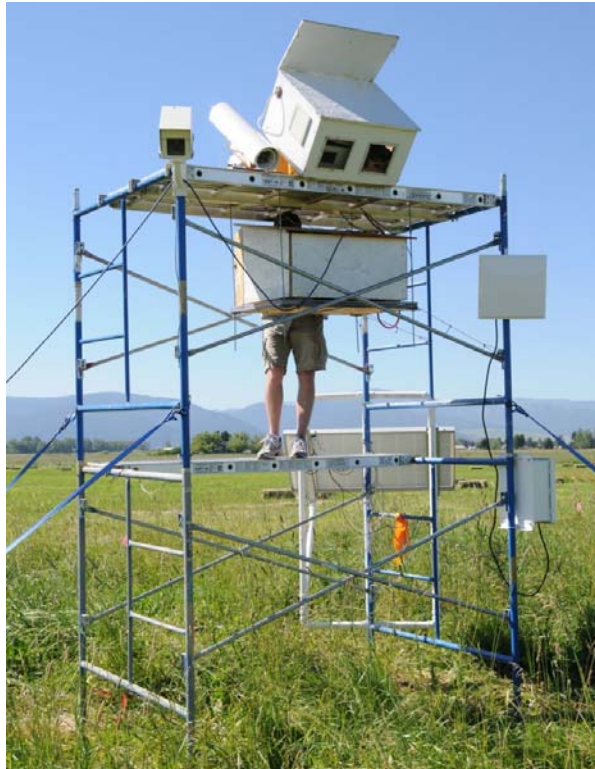
Figure 34. Scaffolding housing the infrared thermal imager (the round tube shaped camera). (J.A.Shaw 2010)
