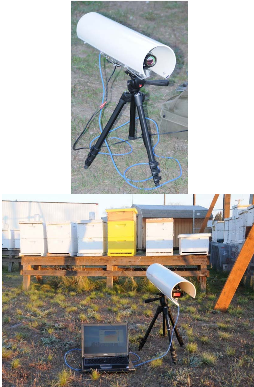
Figure 3: FLIR Photon 320 infrared imager. (J. A. Shaw 2011)
