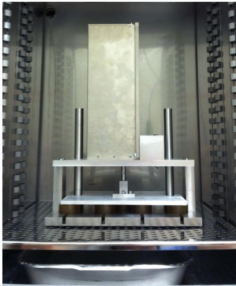
Figure 24: Loading Apparatus inside Incubator
