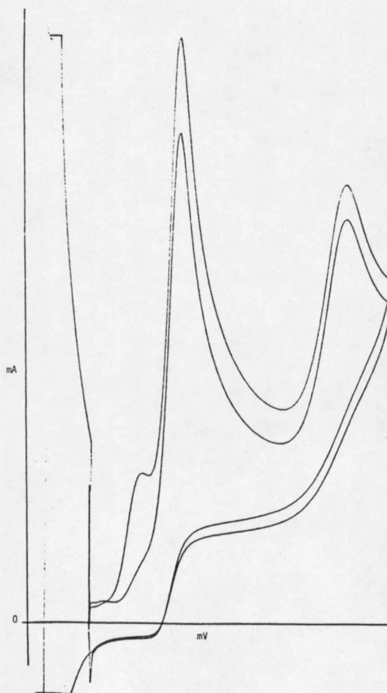
Figure 5. Typical cyclic voltammograms run on "old" instrument. Two consecutive runs of Technizene in TEABr.
