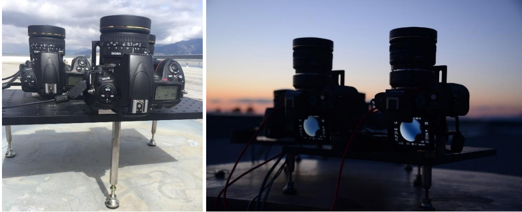
Figure 21. (Left) Nikon D700 three-camera all-sky polarization imaging system recording a cloud phase measurement. (Right) Sony \alpha 7s 3-camera all-sky polarization imaging system during a twilight test conducted to prepare for the 21 August 2017 solar eclipse. (Right) Photo provided courtesy of Joseph A. Shaw.
