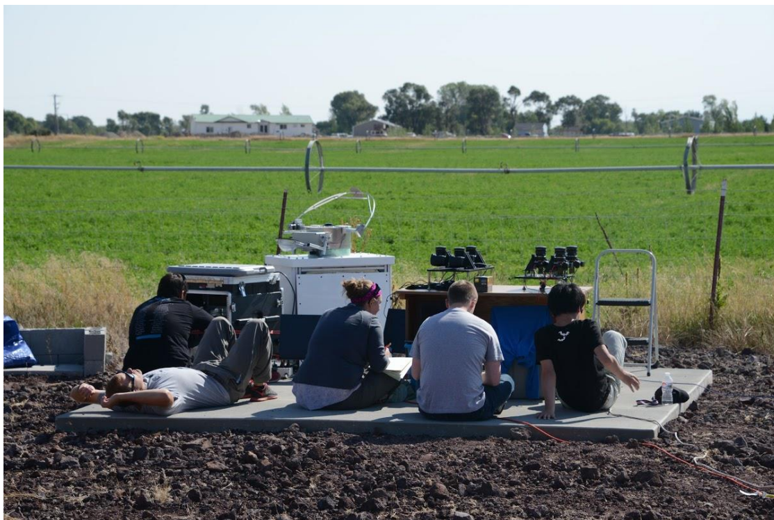
Figure 61. All-sky polarimeters used to measure skylight polarization on 21 August 2017. The LCVR-based all-sky polarimeter is on the left with the two three-camera all-sky polarimeters on the right. The Sony camera system is the closest to the right. Photo provided courtesy of Joseph A. Shaw.
