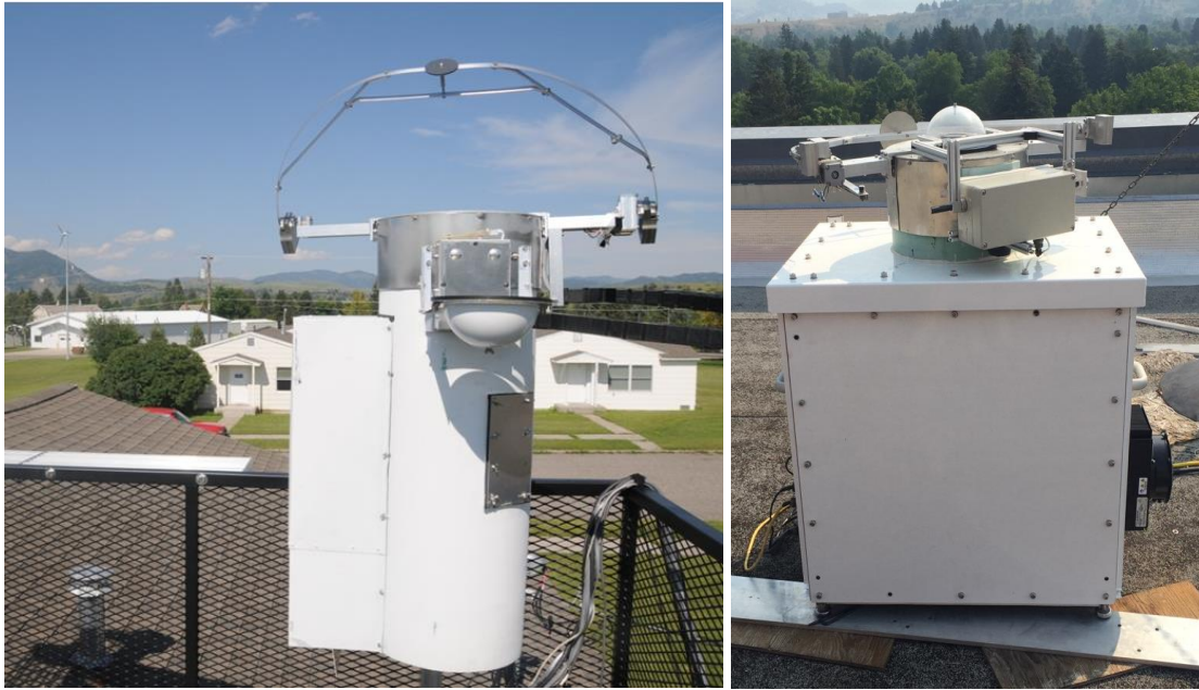
Figure 20. (Left) Old LCVR all-sky polarimeter housing and (Right) new all-sky polarimeter housing.
