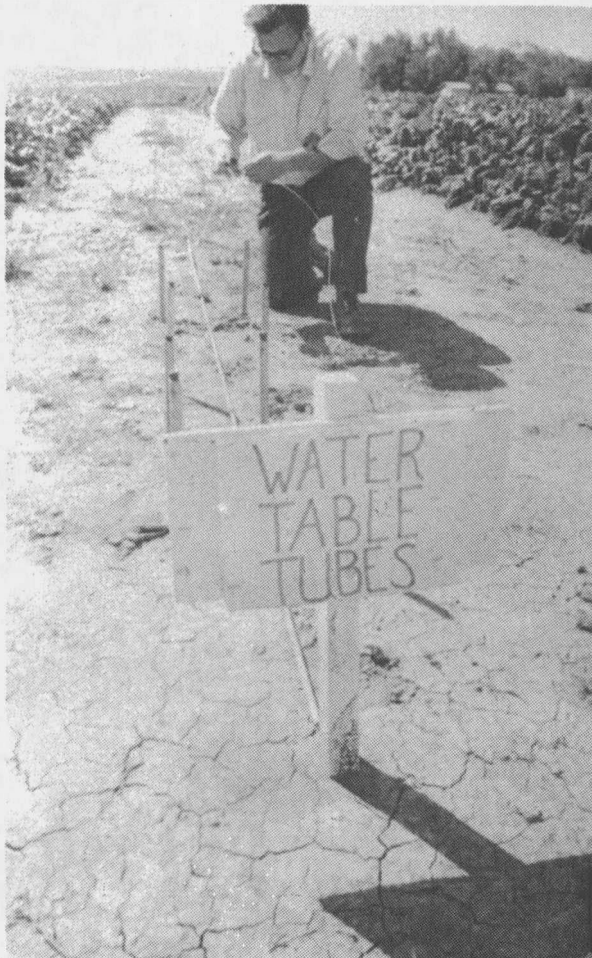
Figure 11. Eight .75-inch outside diameter steel piezometers, installed in one foot increments at soil depths 4- to 11-feet, were used to measure water table depth.
