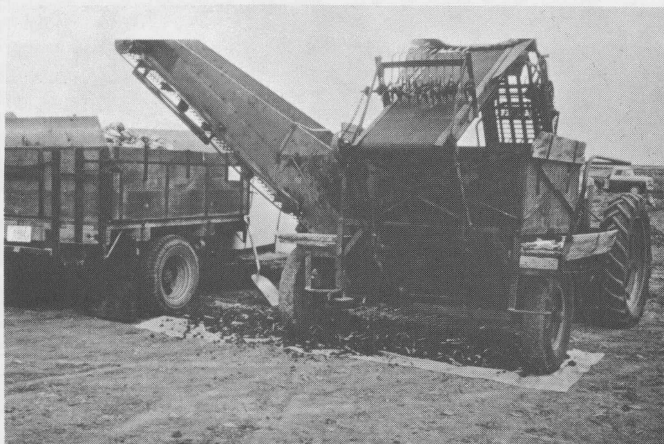
Figure 29. Single row beet digging apparatus. Soil dislodged during transfer of beets into the truck constituted the field tare.
