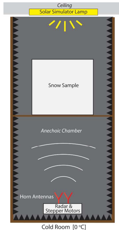
Figure 3. Schematic of laboratory snow melt experiments within an anechoic chamber inside of a cold room with continuous upward-looking polarimetric radar measurements.
